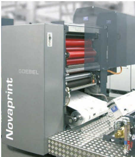
A high capacity web offset press with integrated ink mist exhausting system
