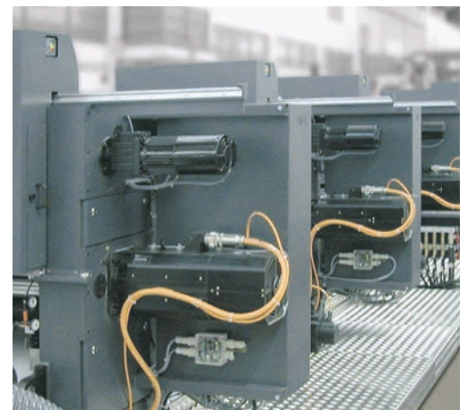
Shaftless drive technology opens up new possibilities for minimizing makeready times and reducing waste
